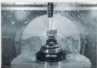
The design of Clean•Tec allows you to wash workpieces and fixtures using coolant – with the machine spindle turned off and the Clean•Tec blades folded! – This enhances the cleaning effect and makes perfect sense if pockets and bores are commonly packed with swarf and chips.
