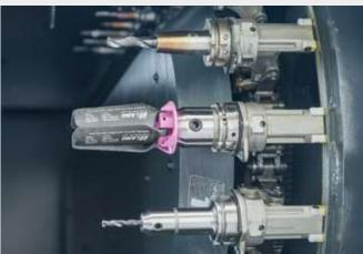
The Clean•Tec Cleaning Fan is stored just like a common tool in the tool magazine and selected automatically via a CNC program. Thanks to its compact design (only  $\emptyset$  68 mm) tool pockets neighboring the Clean•Tec's storage place can be equipped with other tools and don't have to be left empty.
