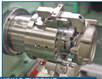
WORKPIECE: HOUSING TURBINE H09M10 0-3021
