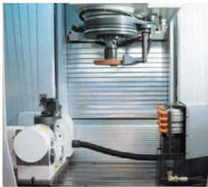
Simultaneous 3 axes control of X, Z & A axis instead of turning.
