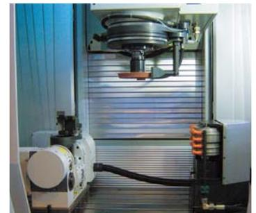
Utilization for 4th and 5th axis rotary table of special grinding centre
