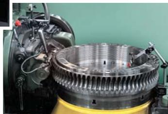
Hobbing of the gears with large module
