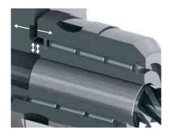
Conventional power chuck high radial transmittable torque unstable / weakened - only limited radial load capacity
