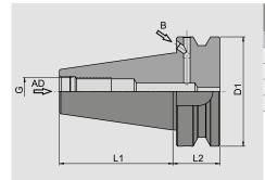
Case-hardened material, hardened and ground Surface hardness: 60-2 HRC Minimum core tensile strength: 950 N/mm² Taper angle tolerance AT<sub>3</sub>
