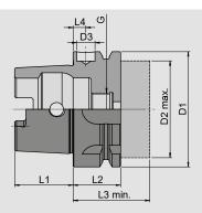
Case-hardened material, hardened and ground Surface hardness: 58-2 HRC Minimum core tensile strength: 1,000 N/mm²
