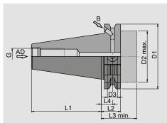
Case-hardened material, hardened and ground Surface hardness: 60-2 HRC Minimum core tensile strength: 950 N/mm² Taper angle tolerance AT<sub>3</sub>
