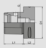
Case-hardened material, hardened and ground Surface hardness: 60-2 HRC Minimum core tensile strength: 950 N/mm²
