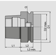
Case-hardened material, hardened and ground Surface hardness: 58-2 HRC Minimum core tensile strength: 1,000 N/mm²
