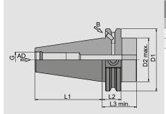
Stock material, hardened, and ground Surface hardness: 60-2 HRC Minimum core tensile strength: 950 N/mm² Taper angle tolerance AT3
