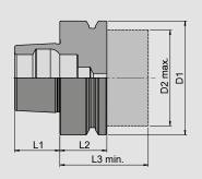
Case-hardened material, hardened and ground Surface hardness: 58-2 HRC Minimum core tensile strength: 1,000 N/mm²
