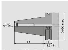
Stock material, hardened, and ground Surface hardness: 60-2 HRC Minimum core tensile strength: 950 N/mm² Taper angle tolerance AT3
