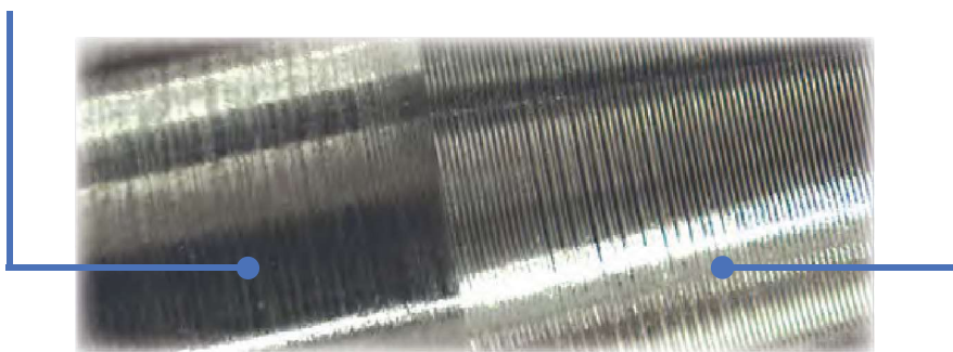
Turned With A multidec® TOP Wiper Insert
