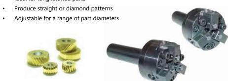
Compact design makes it ideal for use on screw machines and CNC lathes when axial feed knurling from the turret. Parts are self supported and they can extend through the shank for long jobs. We recommend using CONVEX Knurl Dies with this style Knurl Holder. Can also be adapted for burnishing and internal knurling
