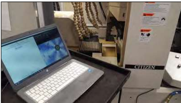
Perfect Zero aligning a micro tool on a Citizen Swiss-style machine
