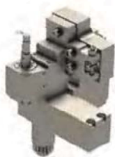
GSH-036-L Gear Hobbing ID Size: Ø3.5mm Output: 3:2 Hobb OD: Ø8mm Hobb Thickness: 12mm Requires 1 tool positions
