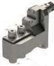
GSE-3607-2D End Drill/Mill Collet Size: ER11 Output: 1:1 Adjustable \pm 30^\circ Double Ended
