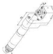
GSE-306-DE512 End Drill/Mill Collet Size: ER11 Output: 1:3 High Speed Double Ended L 4 25 L 4 32
