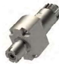
GSC-1310-HP Cross Drill/Mill Collet Size: ER16 Output: 1:1 High Pressure Coolant-Thru Max Pressure 137 Bar G1/8 Fitting [PN#4005-000104] A32 L32
