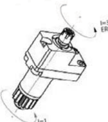
GSE-3307-L-3X End Drill/Mill Collet Size: ER08 Output: 1:3
