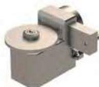
P03-GSP-218 Polygon Milling Arbor Size: \varnothing 8\text{mm} Output: 1:1 Max Tool \varnothing : 45mm Adjustable \pm 2.5^\circ Cutter Offset Machine: P034H
