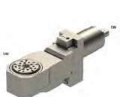
TSUGAMI1-GSW-220 Thread Whirling Ring: Utilis Ring Output: 1:1 Adjustable 0-20° Flight Circle 6mm Machine: S205/S206
