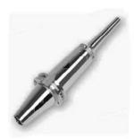
Power Mini Shrink Chuck is perfect for 5-axis-machining in the die & mold and in the medical industry. Very silm at the top like the HAMER Mini Shrink Chuck, the Power Mini Shrink is reinforced at the base. Therefore, efficient milling is possible with an angled tool even at long protruding lengths.
