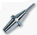
Power Mini Shrink Chuck is perfect for 5-axis-machining in the die & mold and in the medical industry. Very silm at the top like the HAIMER Mini Shrink Chuck, the Power Mini Shrink is reinforced at the base. Therefore, efficient milling is possible with an angled tool even at long protruding lengths.
