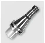
The Power Collet Chuck is designed for the highest cutting performance in High Speed machining. The optimized design with improved construction combines high rigidity with vibration dampening features, giving more protection to the machine, spindle and tool. The universal Power Collet Chuck is a unique high performance chuck that can also be used with standard collets.
