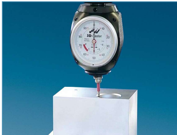
Orientate the machine spindle with the center of a drilled hole or cylindrical O.D.
