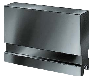
Unstepped jaw BL, unstepped, soft, material 16MnCr5
