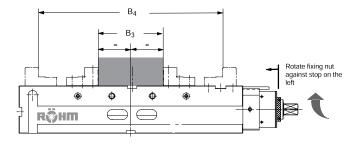
Remove central jaw Fixing nut - stop on the <u>left</u> (spindle rigid) Stroke per jaw: "Z" 53 mm
