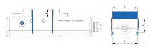
A37 **Draw-down jaws RNG**, with two permanent magnets
