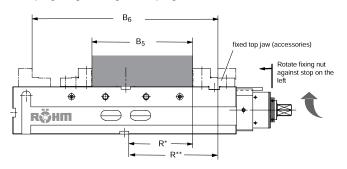
Remove central jaw and movable mounting jaw I.
