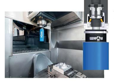
Within the spindle the lubrication impulse is automatically activated. An optimal quantity of Lubriflux lubricant is sprayed to the right place of the tool clamping system.
