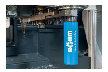
After the lubrication process, Lubritool® is set back to the tool magazine and remains there until the next lubrication cycle.
