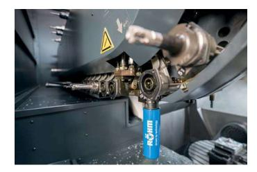
Lubritool® is located in the tool magazine. Whenever the machine control notifies that a lubrication process is necessary, Lubritool® will be set up into the spindle.
