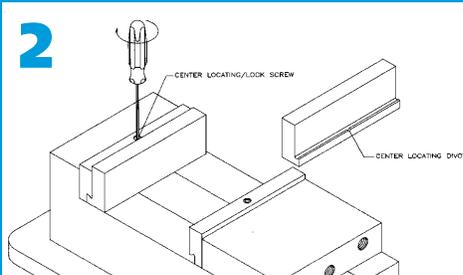
After the accessory is in position simply tighten the provided locking/self-centering screw to secure and locate properly. You are now ready to fixture your workpiece.
