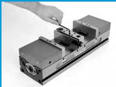
When finished with your job, unlock parallels (if needed) and turn the kick out screw to eject the jaw or parallel. You are ready to repeat the process for your next job.
