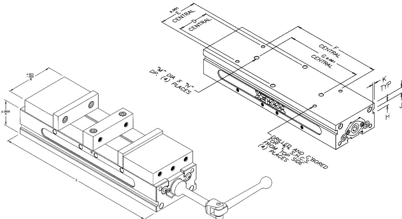
Bodies manufactured from 80,000 PSI ductile cast iron • Ways flame hardened to 40 R/C maximum
