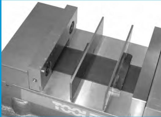
Simply bolt the master jaws to your existing vise. Parallels literally snap in and out for quick set-ups.
