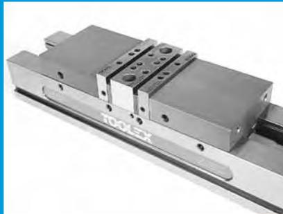
Simply attach the AccuSnap master jaws to the carrier jaw system using the industry standard bolt pattern.
