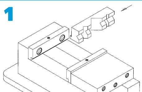
To install the QuickChange System, simply attach the master jaws to your carrier jaw system using the industry standard bolt pattern provided. Align the accessory's gib with the master jaw's dovetail and slide into position.
