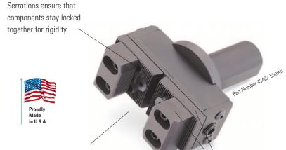
Unit is very easy to use — simply set gap between jaws 1/8" smaller than stock size. As the bar puller slides over the bar along the x-axis, the jaws compress heavy-duty internal die springs to provide high gripping force. The turret then retracts along the z-axis, pulling the bar out to the desired position.
