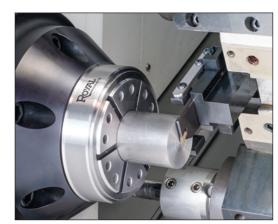
Cycle times are reduced because the turret does not need to index between cut-off and pulling operations.
