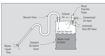
**Heavy Duty Construction** – Entire pump (except ball valve, float and O-ring) is made from either stainless steel or aluminum. Other brands are made from rust-prone carbon steels and light-duty plastics.
