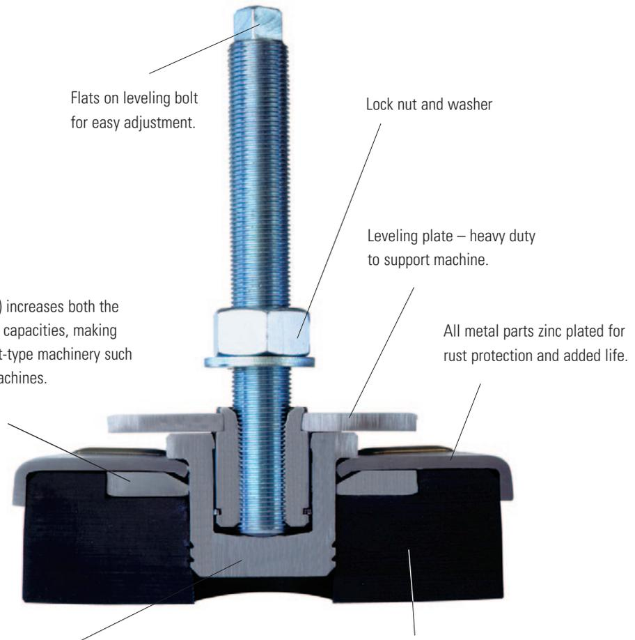
Heavy-duty support cup is machined from a solid steel bar for strength. Other brands rely on a thin drawn cup which often fails by fatigue. Note the increased thickness of the lip and bottom sections.
